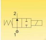
N.O. Normally Open Coil de-energised - Open Coil energised - Closed
